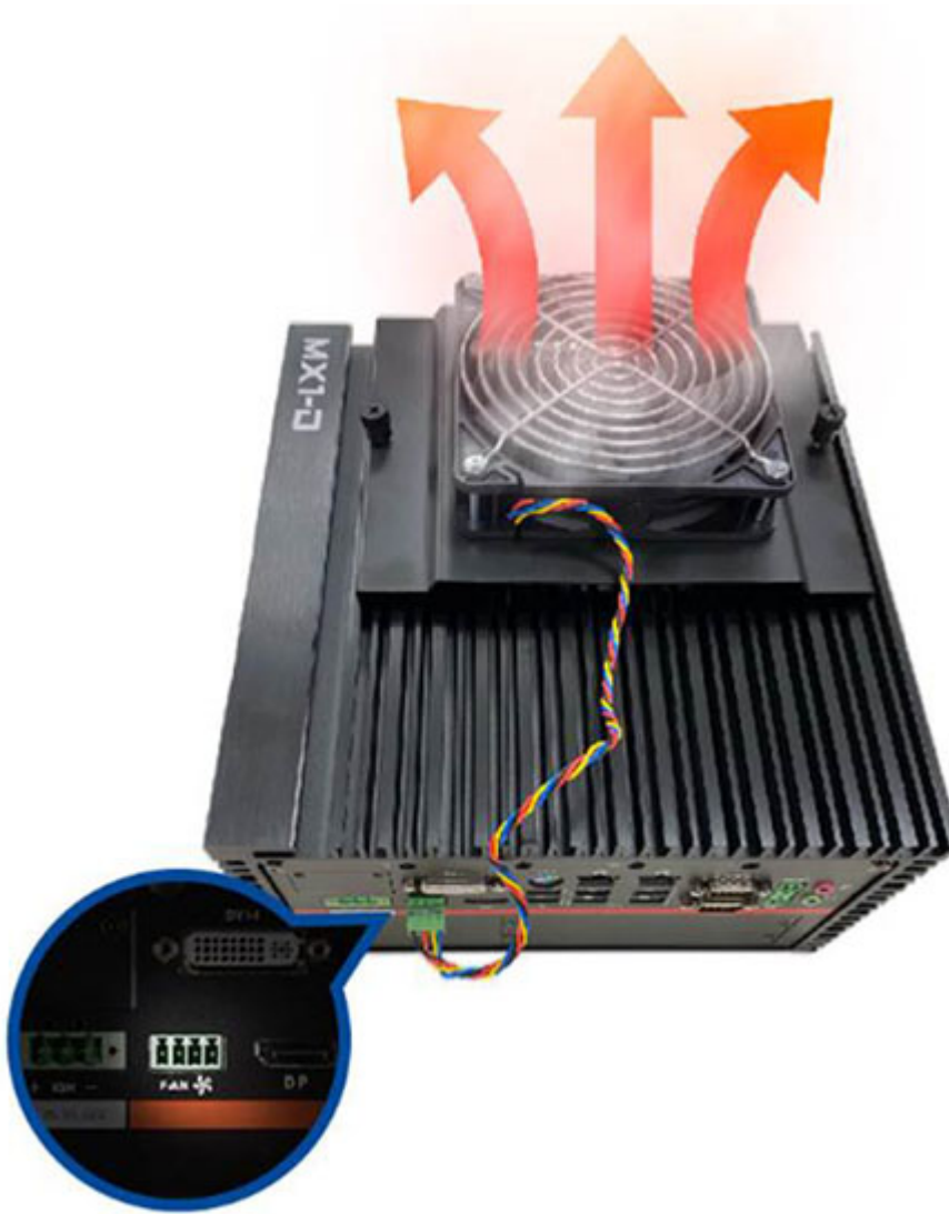
External Fan solution w/ bracket (P/N: 336210000076)
